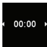
Select the current Time - turn the Control Knob clockwise to select Hour, press the Control Knob to confirm, then turn the Control Knob clockwise again to select the Minutes, press the Control Knob to set.
